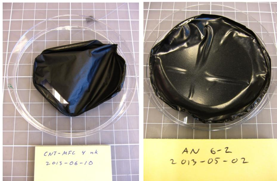
**Figure 1.** Representative pictures of CNT-40 prepared through a) the Linköping University route; b) the Innventia route.
