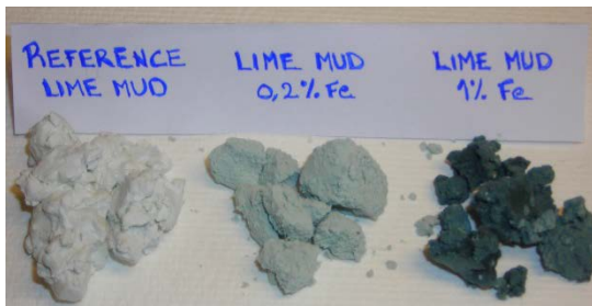
Lime mud samples changing colour upon addition of iron during laboratory causticizing-calcination experiments
