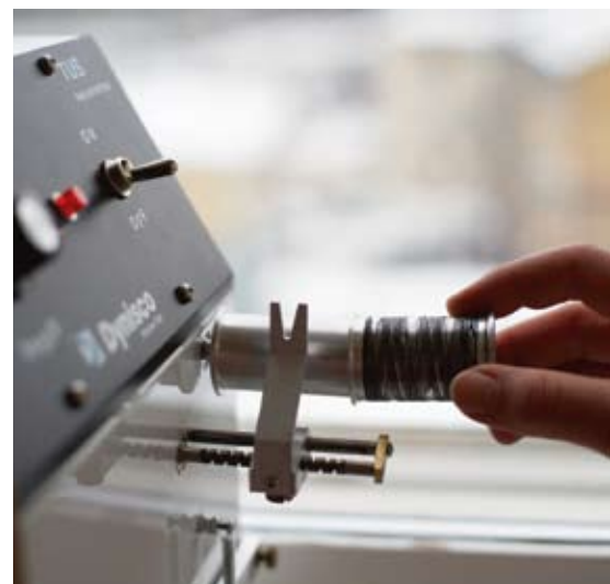
Innventia has invested in equipment for spinning lignin fibre and a furnace for carbonising the fibre. This kiln is also being used for producing activated carbon in another Innventia project.
