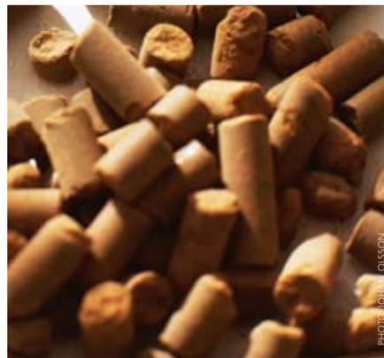
Fortum Värme is investing in a pellet making unit in order to facilitate the handling of lignin fuel.
