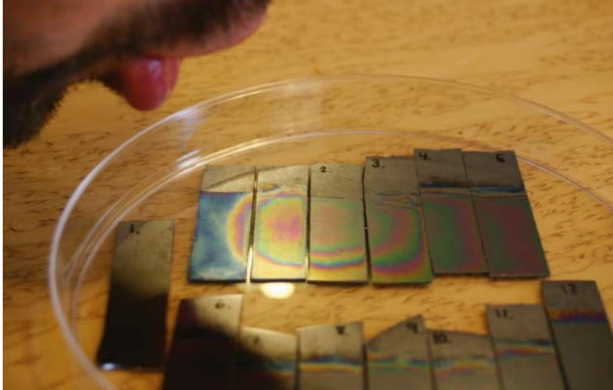
The moisture in exhaled air causes the surface to become coloured, similar to oil on water.
