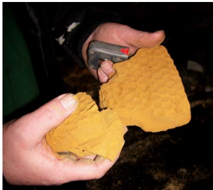
Lignin cake from the demonstration plant.
