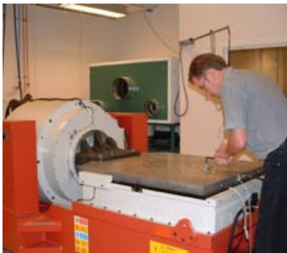
The state-of-the-art equipped Test & Development Laboratory can carry out various environmental tests on packaging materials, packages and products, for resilience to temperature and moisture, vibration, dropping, compression and shunting.
