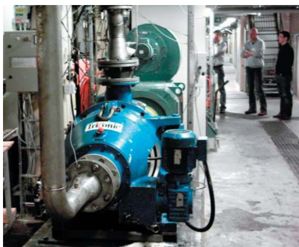
The supplier's equipment, in this case the Pilão Triconic refiner, is used to carry out the trials at STFI-Packforsk.
