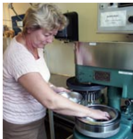
Margaretha Fryklund at the PFI mill. The STFI-Packforsk laboratories for the physical testing of pulp and paper have been accredited with the EN ISO 17025 Certificate.
