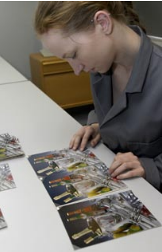
Subjective print evaluation. The HPI Laboratory utilises trained or non-trained test panels to appraise and evaluate print quality.
