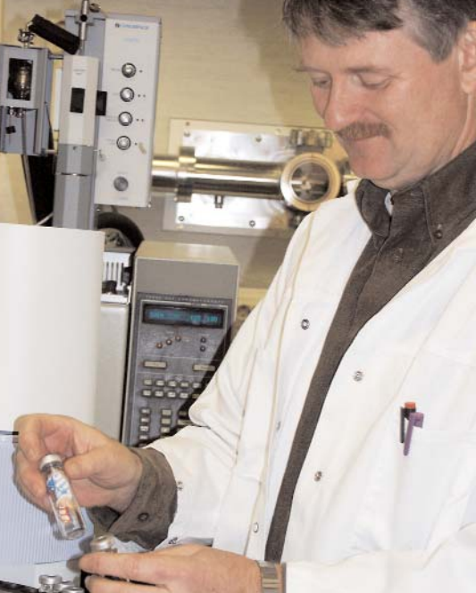
Pierre Ljungquist analyses volatile compounds with headspace GC/MS.
